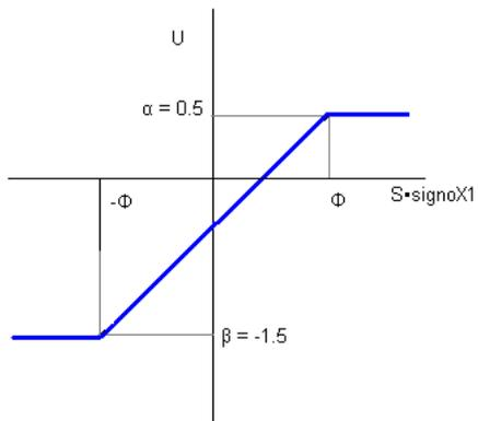
$$u(s) = sat(s) = \begin{cases} -\alpha x_i & \text{cuando } s * signo x_i > \phi \\ -\left(s * \frac{1}{\phi} - 0.5\right) * x_i & \text{cuando } -\phi \leq s * signo x_i \leq \phi \\ -\beta x_i & \text{cuando } s * signo x_i < -\phi \end{cases}$$
